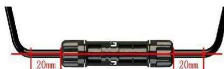
Right way for the cable
